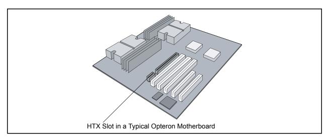
Figure 4-7. HTX Slot
